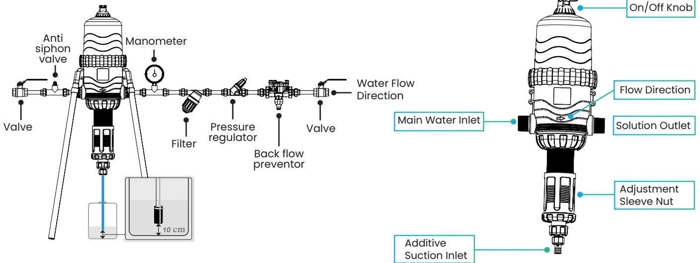
Fig. 2 - Installation illustration
